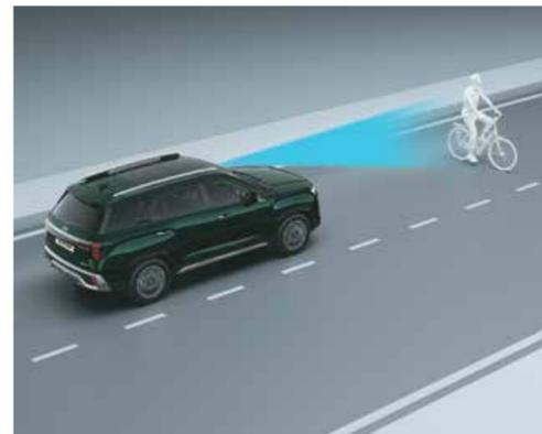
Forward Collision - Avoidance Assist - Cycle (FCA-Cyl)
