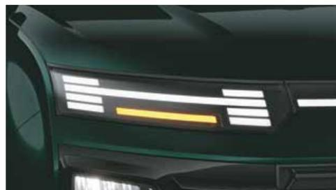
LED turn signal with sequential function
