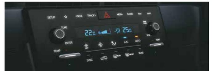
Dual zone automatic temperature control (DATC) with touch control
